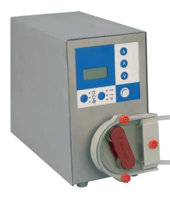
The Peristaltic Dispenser can be supplied with a range of sizes of high strength silicone tubing from 0.8mm bore to 8mm bore, with either a 1.6mm or 2mm wall thickness.
